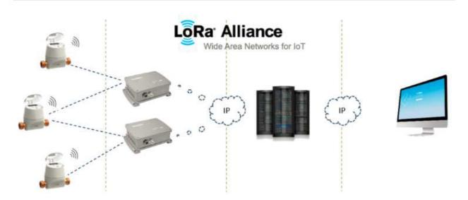
EMR System is a cloud-based smart water meter reading and management system which adopts LoRaWAN Protocol and integrates the water measuring, data transmission, collection, storage and analysis, enabling water utilities as well as water consumers to closely monitor the water usage without additional labor work. It is equipped with an advanced device maintenance function as well, which significantly improves utility/company work efficiency and device management.
